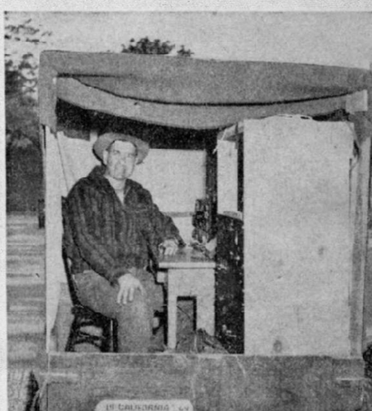
Ingenuity has been an outstanding characteristic of the amateur radio operator. Constantly experimenting to improve his equipment, he has produced many important advances in the electronic art. This "ham" operator showed a talent for improvisation by building an emergency radio station in a small trailer. This station can be hauled quickly to any spot where communication equipment is needed.
